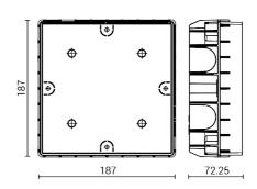
Backbox for wall flush installation, complete with cover
