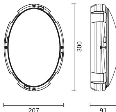
Outdoor luminaire for wall/ceiling installation
