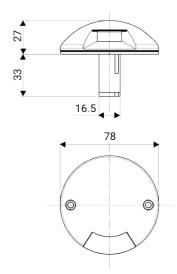
Outdoor walk-over luminaire for ground surface installation
