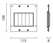
Converging lens with lateral slots for focus regulation
