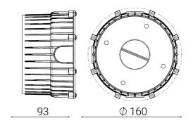
Backbox for wall flush installation, complete with cover
