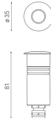
Outdoor ground/wall/ceiling recessed luminaire
