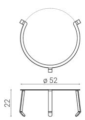
Plasterboard ceiling/wall fixing clip for Ø 52 mm holes
